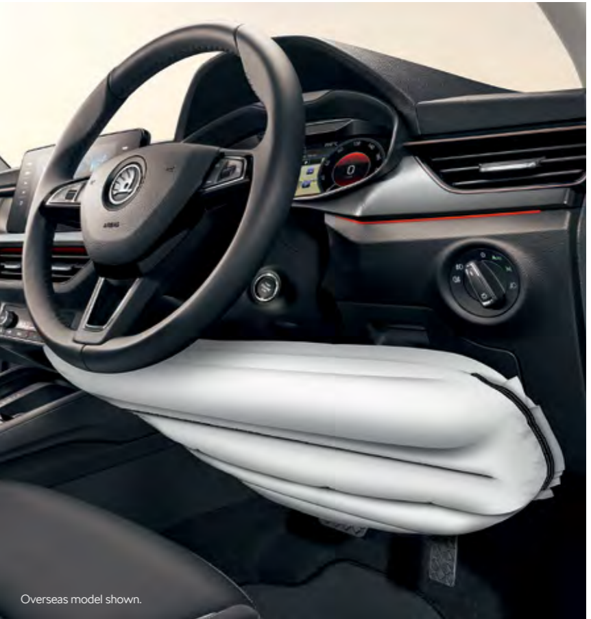
Knee airbag This airbag, which is located under the steering wheel column, protects the driver's knees and shins.
